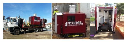
The Track-Truck provides the versatility of having both a small tracked rig, for those hard to get to areas, and the pushing capacity of a 22 tonne truck rig on site at the one time.
